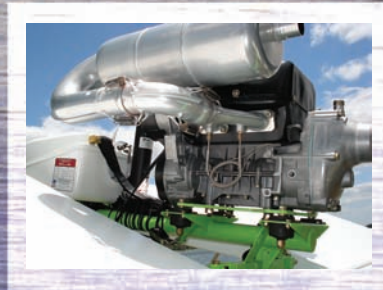
A clean and simple installation of the Rotax 447 engine, showing the hot side here with Jet Hot ceramic coated exhaust pipes.
