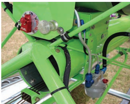
The Andair mini gascolator is shown at the bottom left in this photo. It's the lowest point in the fuel system and where we sample fuel from. The Essex primer and the Andair fuel selector are on panel behind the seat. All three are connected using 3003-0 aluminum tubing and AN fittings.
