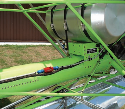
The 5-gallon fuel tank is a cut-down aluminum dune buggy tank. The red device in the fuel line is a 10-micron stainless steel fuel filter.
