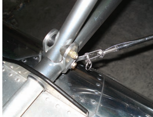
A close-up view of the interface of the main strut to the float. The U-shaped bracket was borrowed from the powered parachute industry. All components are anodized.
